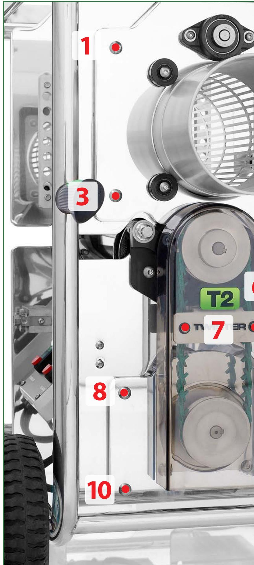
Figure 2.3 Tumbler adjustment and belt replacement
