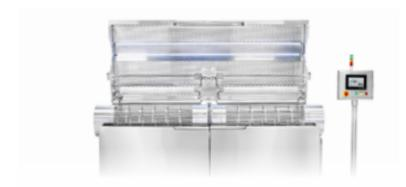
**Blade Drive Motor: 20HP** Tumbler Motor: 1HP **Blower Motor: 25HP**
