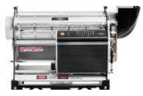
Product Number: 24-9019-00-P Input Voltage: 115V, 60 Hz Current Draw: 2.5A Blade Motor: 1/4HP, 200W Cut Height: .040in / 1mm Tumbler Diameter: 5in / 10.1cm Tumbler Slots: 40 x .25in/.6cm Weight: 56lbs /25.4kg Shipping Weight (w/ T4-LC): 120lbs / 54.4kg Length: 25in / 63.5cm Width: 15in / 38.1cm Height: 16.5in / 42cm Circuit Breaker Required: 15A / 120V Throughput: 23lbs/hr wet, 16lbs/hr dry
