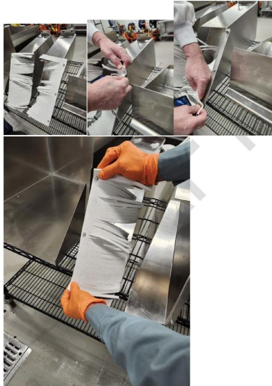
Figure 8.3: Curtain orientation — convex side inward
